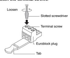
\* The following explanation uses a Euroblock plug that features a tab as an example.
