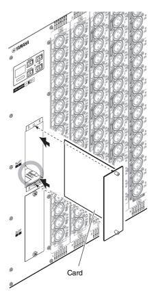
**4.** Fasten the card using the screws attached to the card.
