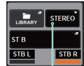
L/R PATH pull-down menu in the SELECTED CHANNEL VIEW screen
