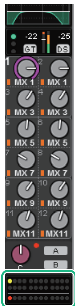
DCA/MUTE ASSIGN field on the OVERVIEW screen
