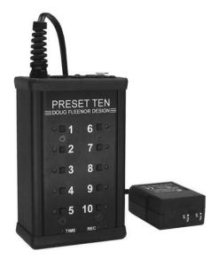
The *Preset 10 Portable* can act as a seamless backup for DMX512 lighting consoles or as a stand-alone DMX512 preset console. The *Preset 10 Portable* is capable of storing up to ten presets. These presets are recorded by capturing the output of a DMX512 console. Each preset can be assigned a unique crossfade time, from 0 to 999 seconds. Presets are recalled by pressing one of the buttons.
