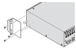
**2** Remove the 2 screws that secure the handle, and remove the handle.
