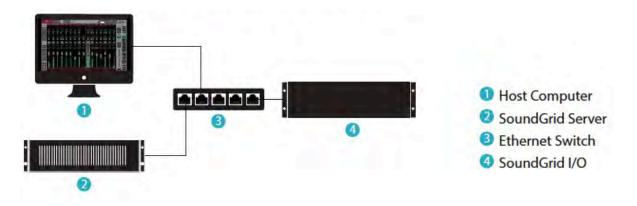
Maximum distances between devices vary depending on configuration. However, maximum cable length between I/Os and switch is usually 100 meters. When connecting the Ethernet cable to an STG-2412, make sure that the connectors and the cable are protected from stage equipment and traffic. For SoundGrid protocol cable and switch specifications, visit the Waves Support desk: http://www.waves.com/support.
