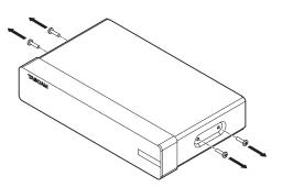
2. Align the included attachment brackets with the enclosure.
