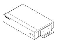
**3.** Use the four removed screws to install the attachment brackets on the unit.
