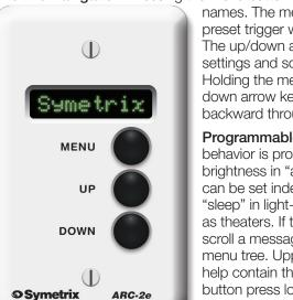
names. The menu button also acts as a preset trigger when a preset list is scrolled. The up/down arrow buttons adjust parameter settings and scroll through preset lists. Holding the menu button and using the up/down arrow keys moves you forward or backward through the menus.
