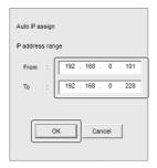
IP addresses in the specified range are assigned to the remote controllers automatically.
