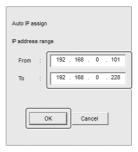
IP addresses in the specified range are assigned to the cameras automatically.
