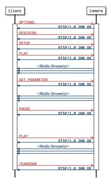
The RTSP "GET\_PARAMETER" method in the sequence above is used to keep the RTSP streaming alive. You can pause the streaming by using PAUSE command after starting live streaming by using PLAY command. To resume, send PLAY command again. The cameras resume video streaming at the current point by forcing IDR frame insertion at the point of reception of PLAY resume request. Videos before the pause and after the resume are not in sequence.
