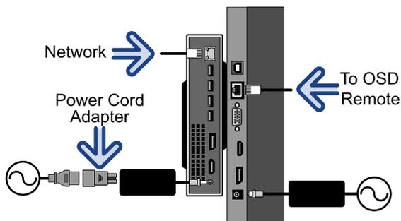
**Note:** It is recommended that you always connect the AC Power Adapter to the device before connecting to Mains Power.
