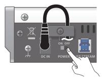
Turn on the power in the order of source devices → output devices.
