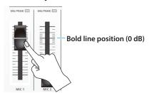
2. Move the [MAIN] knob to a position near the indicator (0 dB).
