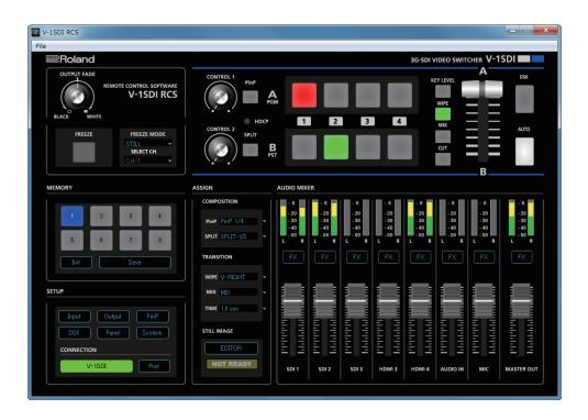
V-1SDI RCS is software designed to control the V-1SDI remotely using a computer.
