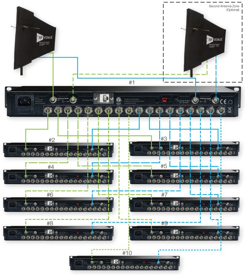
\*DISTRO9HDR #1 (Master) can feed signals to up to 9 additional DISTRO9HDRs. Each connected DISTRO9HDR can feed up to 9 receivers.
