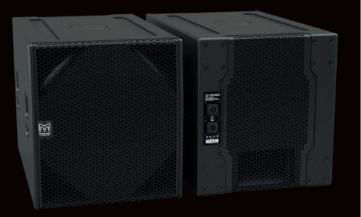
Designed for touring sound and installations, the SXC115 is a compact, high performance cardioid subwoofer. It features a 15" (380mm) forward facing driver and a 12" (300mm) rear facing driver, each driven independently by separate amplifier channels and DSP. Each driver has its own chamber with optimised bass reflex porting.
