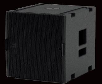
The SXF115 is a passive subwoofer designed to extend the performance of Martin Audio WPM and MLA Mini systems down to 42Hz. Featuring a powerful, long-excursion 15" (380mm)/4" (100mm) voice coil driver in a very compact bass reflex enclosure, it can be flown as part of a WPM or MLA Mini array, or ground-stacked separately.
