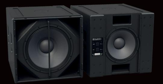
Designed for touring sound and installations, the SXC118 is a compact, high performance cardioid subwoofer. It features an 18" (460mm) forward facing driver and a 14" (356mm) rear facing driver, each driven independently by separate amplifier channels and DSP. Each driver has its own chamber with optimised bass reflex porting.
