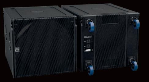
The SXCF118 is a compact, high performance cardioid subwoofer. The flown version of the SXC118, it is the ideal partner for flown WPS arrays — combining maximum low frequency output with pattern control. It features an 18" (460mm) forward facing driver and a 14" (356mm) rear facing driver, each driven independently by separate amplifier channels and DSP. Each driver has its own chamber with optimised bass reflex porting.
