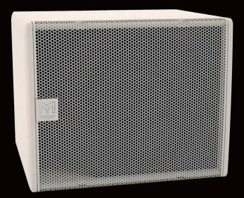
The SX112 is an ultra-compact direct radiating sub-bass system designed to extend the bandwidth and increase the headroom of full-range loudspeaker models. It features a very efficient 12" (300mm) long-throw bass driver with a high power 3" (75mm) voice coil and generously-sized reflex ports for low noise, high power operation.
