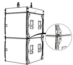
Repeat the procedure for each sub to be included in the array to a maximum of 16 SXCF118. For arrays that consist of SXCF118 and WPS, please refer to the WPS manual.
