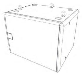
Remove the M10 counter-sunk screws and screw the eyebolts into position. We would recommend three eyebolts and an additional eyebolt as a redundant safety bond. This should be attached to a different point than the other bolts to support the cabinet in the event of the other points failing.
