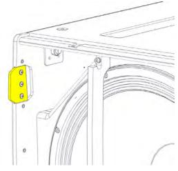
Replace the grill supports and fit the grille making sure the safety screws are used.\
