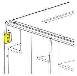
Replace the grill supports and fit the grille making sure the safety screws are used.
