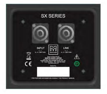
The SX110 has a pair of NL4 connectors on the rear panel. These are wired in parallel and whilst one is nominally labelled 'INPUT' and the other as 'LINK', connection in and out can be made to either connector. Connection to the drive unit(s) is made to pins 1+/-. There is no internal connection to pins 2+/- although these are linked together so can be used for example to carry a mid/top signal and connected to a full range system using a cable wired with reverse connections (pins 2 to pins 1).
