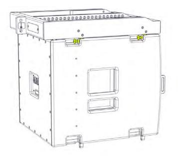
If more subs are to be linked under the first, raise the height of the first sub so you can position a second sub directly under the first. Remove the flying pins in the bottom drop-down rigging links in the first sub and lower it onto the second ensuring that the rigging links engaging all four rigging slots in the second sub exactly as you did with the frame and first cabinet.
