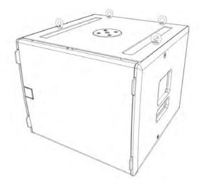
Remove the M10 counter-sunk screws and screw the eyebolts into position. We would recommend four eyebolts and an additional eyebolt as a redundant safety bond. This should be attached to a different point than the other bolts to support the cabinet in the event of the other points failing.
