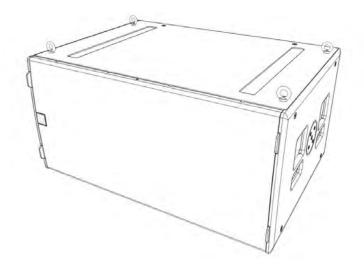
Remove the M10 counter-sunk screws and screw the eyebolts into position. We would recommend four eyebolts and an additional eyebolt as a redundant safety bond. This should be attached to a different point than the other bolts to support the cabinet in the event of the other points failing.
