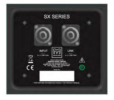
The SX212 has a pair of NL4 connectors on the rear panel. These are wired in parallel and whilst one is nominally labelled 'INPUT' and the other as 'LINK', connection in and out can be made to either connector. Connection to the drive unit(s) is made to pins 1+/-. There is no internal connection to pins 2+/- although these are linked together so can be used for example to carry a mid/top signal and connected to a full range system using a cable wired with reverse connections (pins 2 to pins 1).
