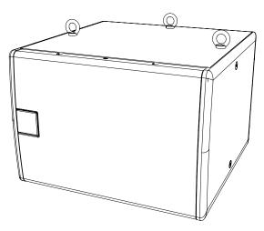
Remove the M8 counter-sunk screws and screw the eyebolts into position. We would recommend three eyebolts and an additional eyebolt as a redundant safety bond. This should be attached to a different point than the other bolts to support the cabinet in the event of the other points failing.
