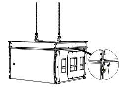
Remove the pins from the stow position, rotate the links to line up with the pin hole position on the SXHF218 above.
