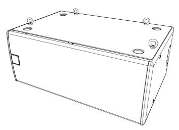
Remove the M8 counter-sunk screws and screw the eyebolts into position. We would recommend four eyebolts and an additional eyebolt as a redundant safety bond. This should be attached to a different point than the other bolts to support the cabinet in the event of the other points failing.
