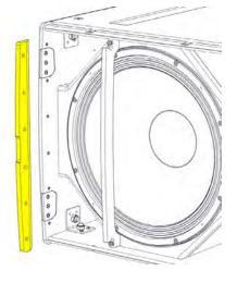
Remove the three screws from the bracket.
