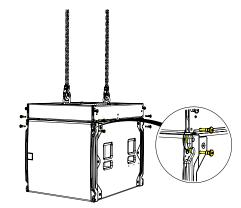
Raise the WPSGRIDt and SXCF118 to a height suitable to fit another SXCF118 below the array, lower it making sure the protective nylon skids line up and fit into the recessed channels on the SXCF118 below.
