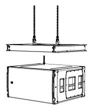
Replace the WPLGRIDt pins to link the SXHF218 securely to the WPLGRIDt. The SXHF218 pins for the first cabinet are not needed in this configuration and can be placed back in the stowed position.
