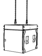
Replace the pins to link and lock the SXCF118 securely to the WPSGRIDt.
