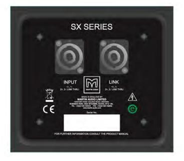
The SX210 has a pair of NL4 connectors on the rear panel. These are wired in parallel and whilst one is nominally labelled 'INPUT' and the other as 'LINK', connection in and out can be made to either connector. Connection to the drive unit(s) is made to pins 1+/-. There is no internal connection to pins 2+/- although these are linked together so can be used for example to carry a mid/top signal and connected to a full range system using a cable wired with reverse connections (pins 2 to pins 1).
