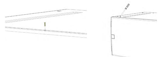
Remove the screws from the grille support on the side of the cabinet and remove the grille support.
