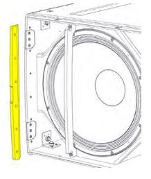
Remove the three screws from the bracket.
