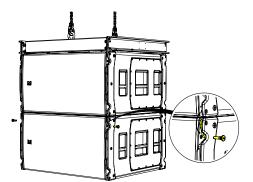
Remove the 4 link pins from the WPLGRIDt and also remove the 4 pins from the from SXHF218 to release the links. Rotate the SXHF218 links and line them up with the pin holes in the WPLGRIDt.
