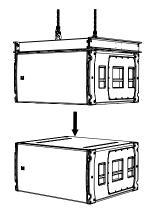
Replace the pins into the lock position on the cabinet above making sure all four links are securely attached. Repeat the process until the correct amount of SXHF218's are flown, the maximum number is 16 SXHF218.
