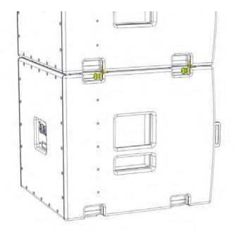
More cabinets can be added as required or transition frames connected to enable flying of either MLA Mini or WPM arrays under the SXP115. For more details see the User Guides for MLA Mini and WPM.
