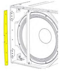
Remove the three screws from the bracket.
