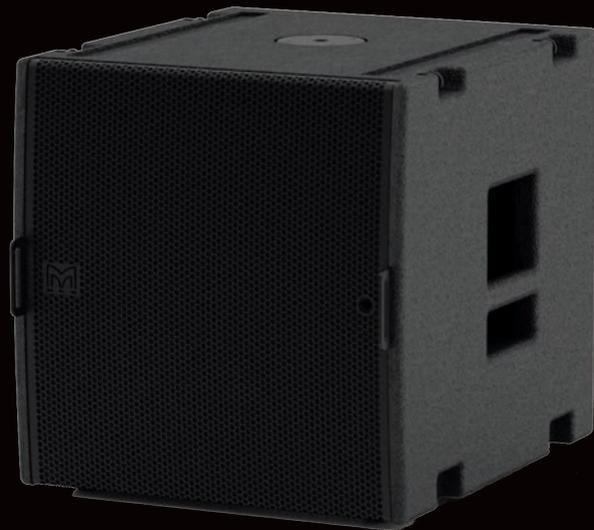
The SXF115 is a passive subwoofer designed to extend the performance of Martin Audio WPM and MLA Mini systems down to 42Hz. Featuring a powerful, long-excursion 15" (380mm)/4" (100mm) voice coil driver in a very compact bass reflex enclosure, it can be flown as part of a WPM or MLA Mini array, or ground-stacked separately.
