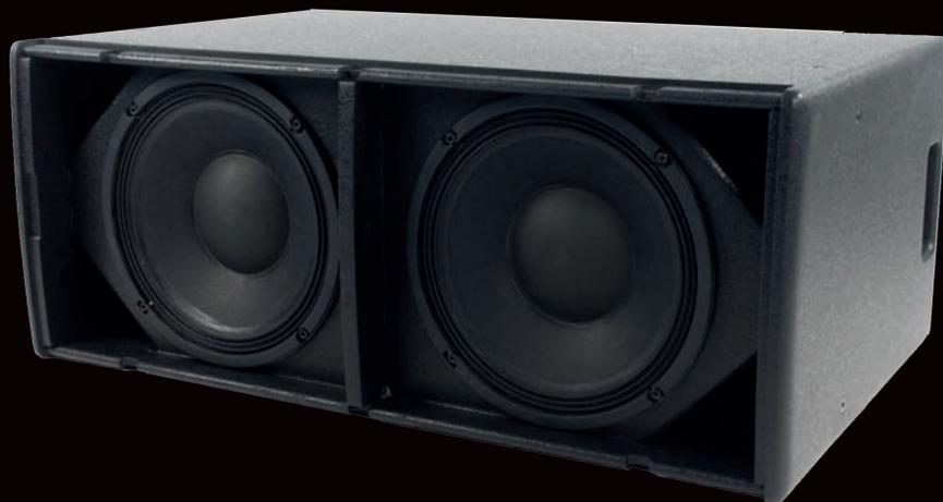
The SX210 is a slimline dual-driver subwoofer designed for situations that call for a visually unobtrusive enclosure. It can be used singly, stacked or flown via integral M8 inserts and its ultra-compact size makes it ideal for applications where space is limited. It features dual 10" (250mm)/2" (50mm) voice coil drivers and generously sized low frequency ports for reduced air noise.
