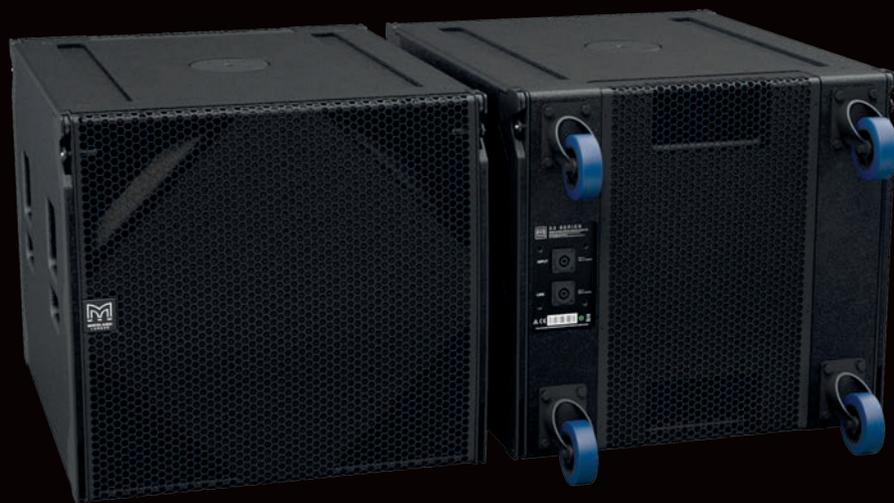
The SXCF118 is a compact, high performance cardioid subwoofer. The flown version of the SXCF118, it is the ideal partner for flown WPS arrays — combining maximum low frequency output with pattern control. It features an 18" (460mm) forward facing driver and a 14" (356mm) rear facing driver, each driven independently by separate amplifier channels and DSP. Each driver has its own chamber with optimised bass reflex porting.
