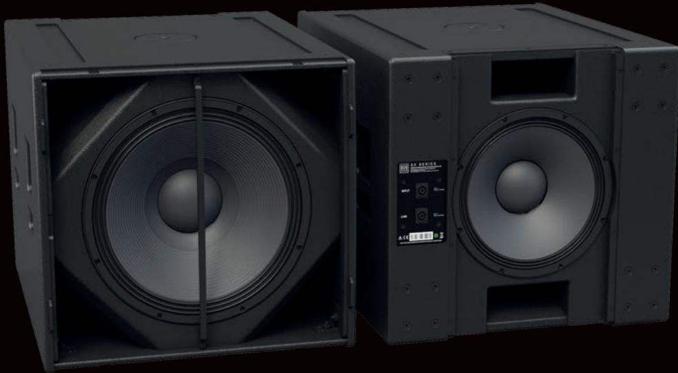
Designed for touring sound and installations, the SXC118 is a compact, high performance cardioid subwoofer. It features an 18" (460mm) forward facing driver and a 14" (356mm) rear facing driver, each driven independently by separate amplifier channels and DSP. Each driver has its own chamber with optimised bass reflex porting.
