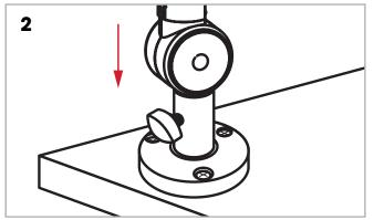
Insert the arm into the hole in the top of the surface mount desk insert.
