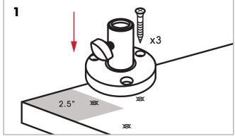
Place surface mount at least 2.5" from the edges of the desk. Then, use a screw driver to secure the surface mount.
