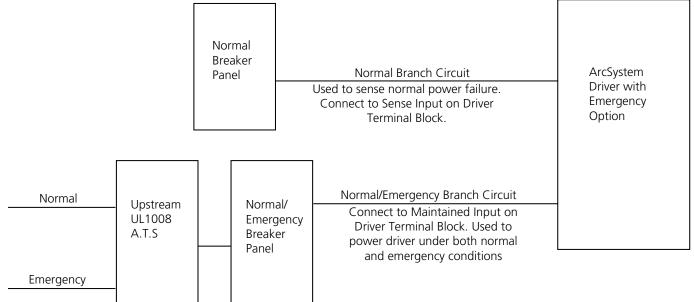
If normal power to the sense input is lost, the driver will force the luminaire on at 100% overriding all other control signals. There is no control of the driver/luminaire via wireless ArcMesh or wired DMX until normal power is restored at the sense input.
