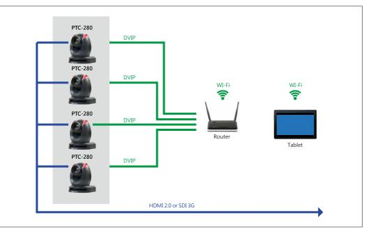
The camera control app is able to control datavideo PTZ cameras. Once you install the app on the tablet, easy to control the cameras in the same network!
