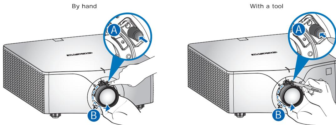
6. Remove the lens through the front of the projector.
