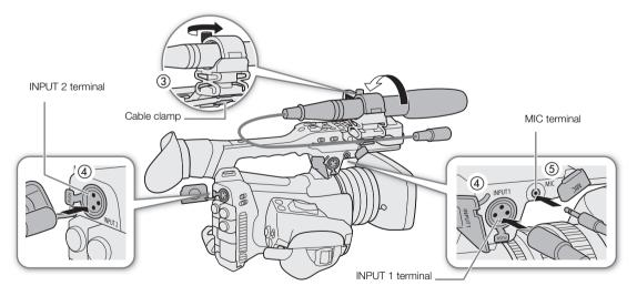
Using the INPUT 1/INPUT 2 terminals, you can record audio independently from a microphone or audio input source.
