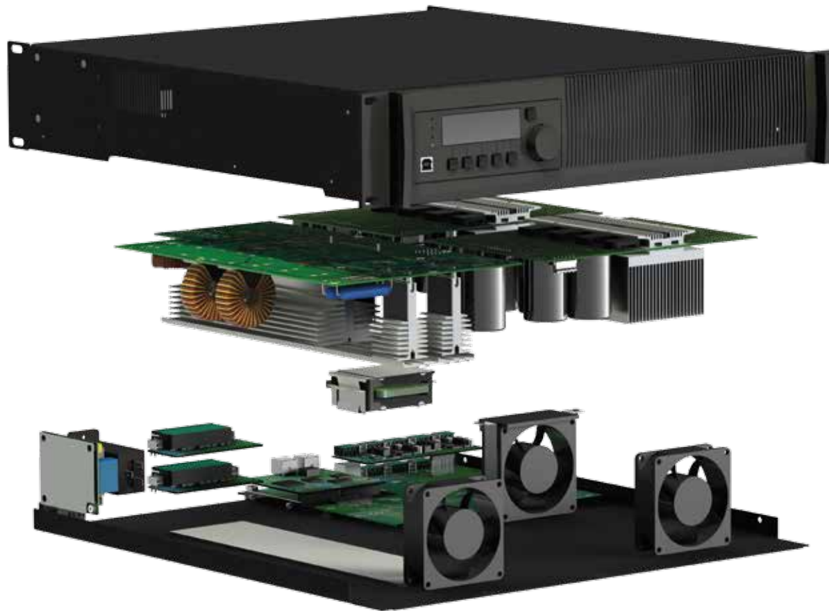
PowerMatch amplifier, internal view
