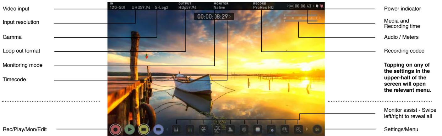
The Shogun Studio 2 is controlled by a simple user-friendly touchscreen interface. Pictured above is the home screen and main controls seen when the Shogun Studio 2 is attached to a compatible input. Touching the icons/text will open menus for the relevant functions.
