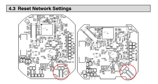
Jumper link **CN9** on the main PCB board lets you reset the network settings to factory default. To reset, short the link for 10s whilst applying power to the unit.
