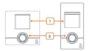
**LCD Display** – Colour display providing information on the selected channel or output mix. It can also display a Source or Scene list when the rotary is pressed if such function is assigned to the IP1.
