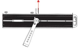
2. Unscrew the retainer screw from the Gobo Holder.
